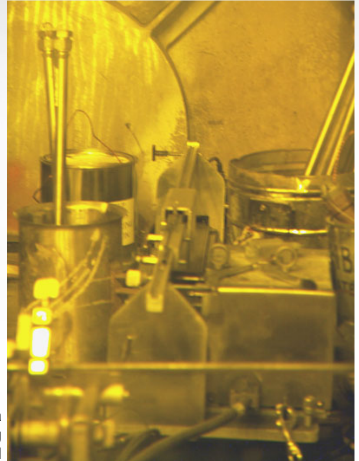
Longitudinal slitting of a tritium-producing burnable absorber rod
